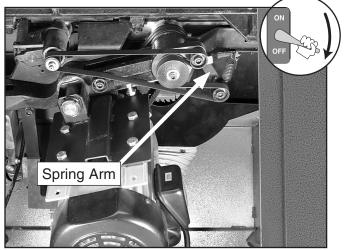
Figure 82. Scoring blade belt tension arm.
